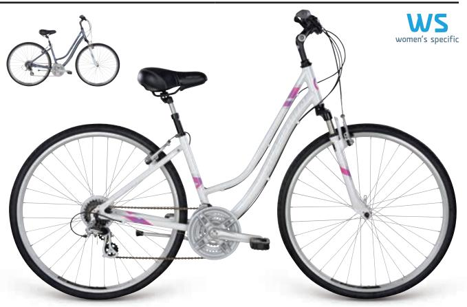
700c Low step through alloy frame with comfort geometry.
