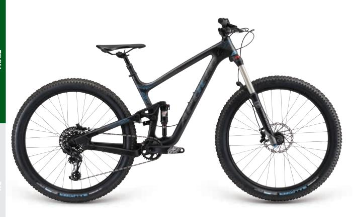
New 27.5" plus carbon dual suspension, 130mm travel, Boost 148mm
