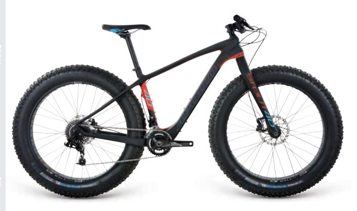
Apollo's carbon fat frame tapered head tube, with 12mm thru axle rear
